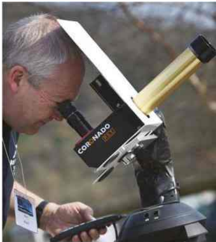
▲ A Coronado PST is a compact, portable and affordable solar telescope
